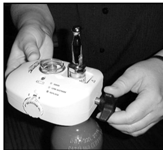
FIGURE F Attaching the OXYMATIC 400 Series conserver to the cylinder
